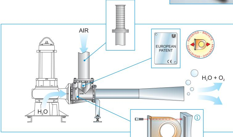
The OXYGEN 80, 100 and 150 ejectors are characterised by the presence of an interchangeable diaphragm covered in corrosion resistant polyurethane material (Vulkollan), which is fixed by two nuts which can be easily replaced and which makes the initial calibration of the system or any maintenance work much easier.
